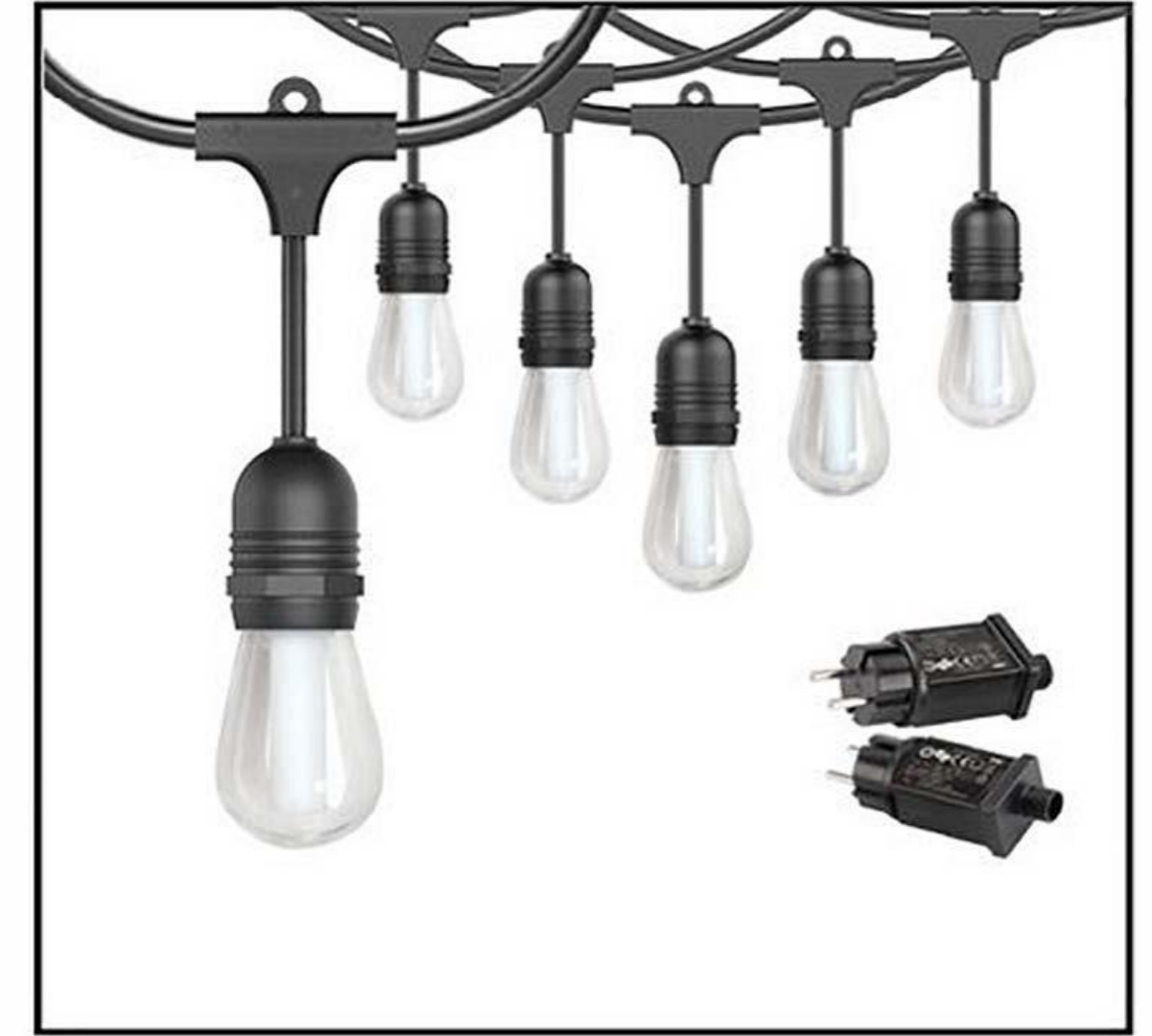
Product Model: LD-12-24FT-S14/F-P/C/C-Warm White 12CT 24FT LED S14 Low voltage decoration Flame Effect String Light(Transparent Plastic Blister/ Warm White SMD LED) Bulb Type Included: SMD LED Material: Plastic Power: S14 0.4W/Bulb(Warm White) Wire:VDE H05VV-F 0.5mm 2 /2C Black Wire Voltage: AC220-240V 5V 6W Function: 1.Flame effect;2.Always bright warm white
