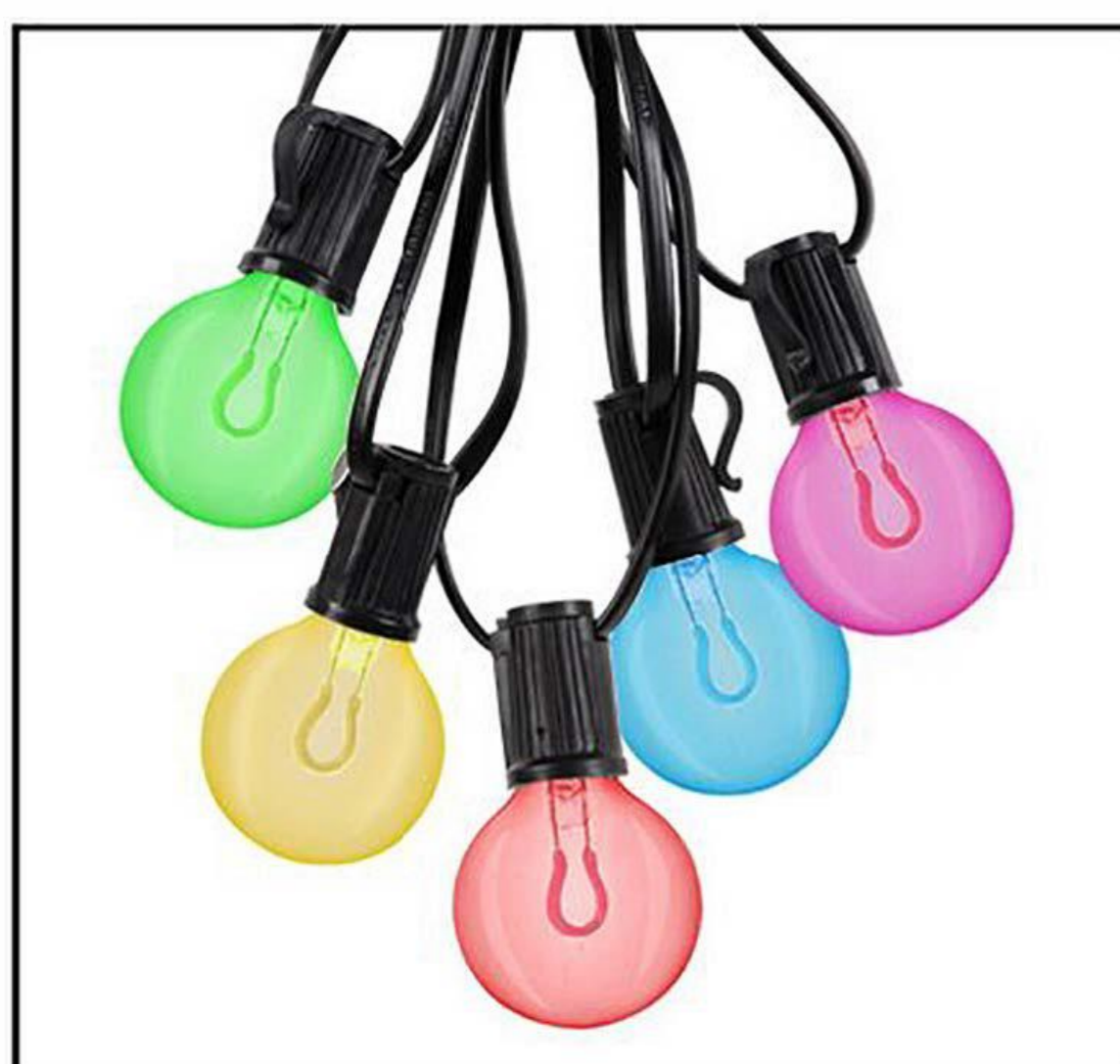
Product Model: LD-25-25FT-E17/G50/H-P/C/Mu-Multi color 25CT 25FT LED E17 G50 String Light- (Transparent Plastic Multi color Blister/ Multi color Filament LED) Bulb Type Included: Filament LED(Flexibility) Material: Plastic Base/Socket: E17 Power: 0.4W/Bulb Wire: SPT-1 20AWG/2C Black Wire Lamp distance: 6"x12"x6" Voltage: 120V
