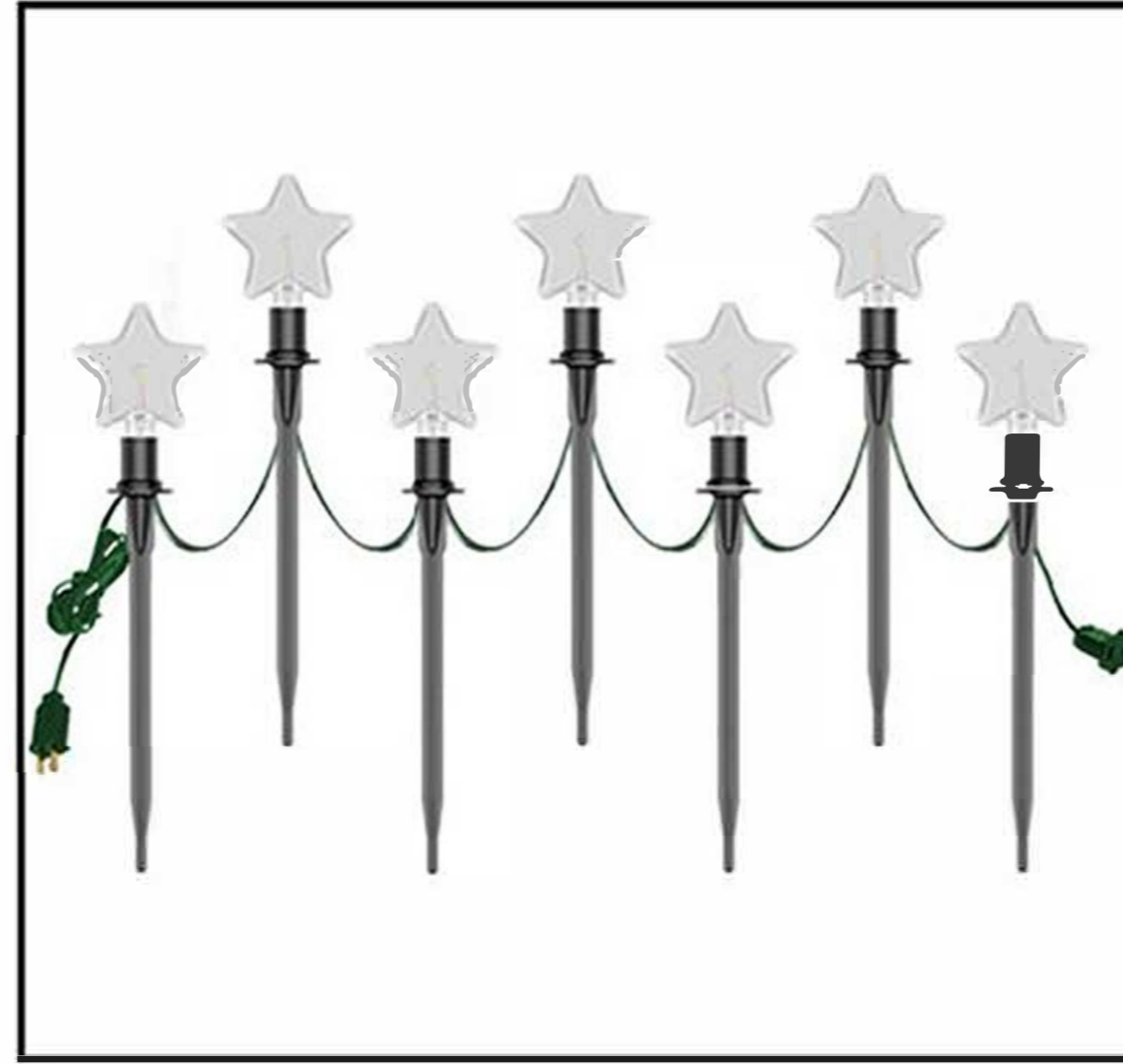
Product Model: LD-7CT-12FT-E17/Star/LED-W/G-Warm White 7CT 12FT LED E17 Christmas star shape frosted ground plug lamp (shape frosted Plastic Blister/ Warm White Filament LED) Bulb Type Included: Filament LED Material: Plastic Base/Socket: E17 Power: 0.4W/Bulb Wire: SPT-1 20AWG/2C Green Wire Lamp distance: 30"x18"x6" Voltage: 120V
