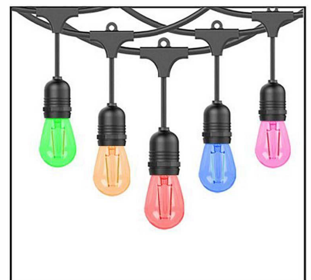
Product Model: LD-15-48FT-E26/S14/T-P/C/Mu-Multi color 15CT 48FT LED E26 S14 String Light- (Transparent Multi color Plastic Blister/ Multi color Filament LED) Bulb Type Included: Filament LED Material: Plastic Base/Socket:E26 Power: 2W/Bulb Wire:SJTW 18AWG/2C Black Wire Voltage: 120V
