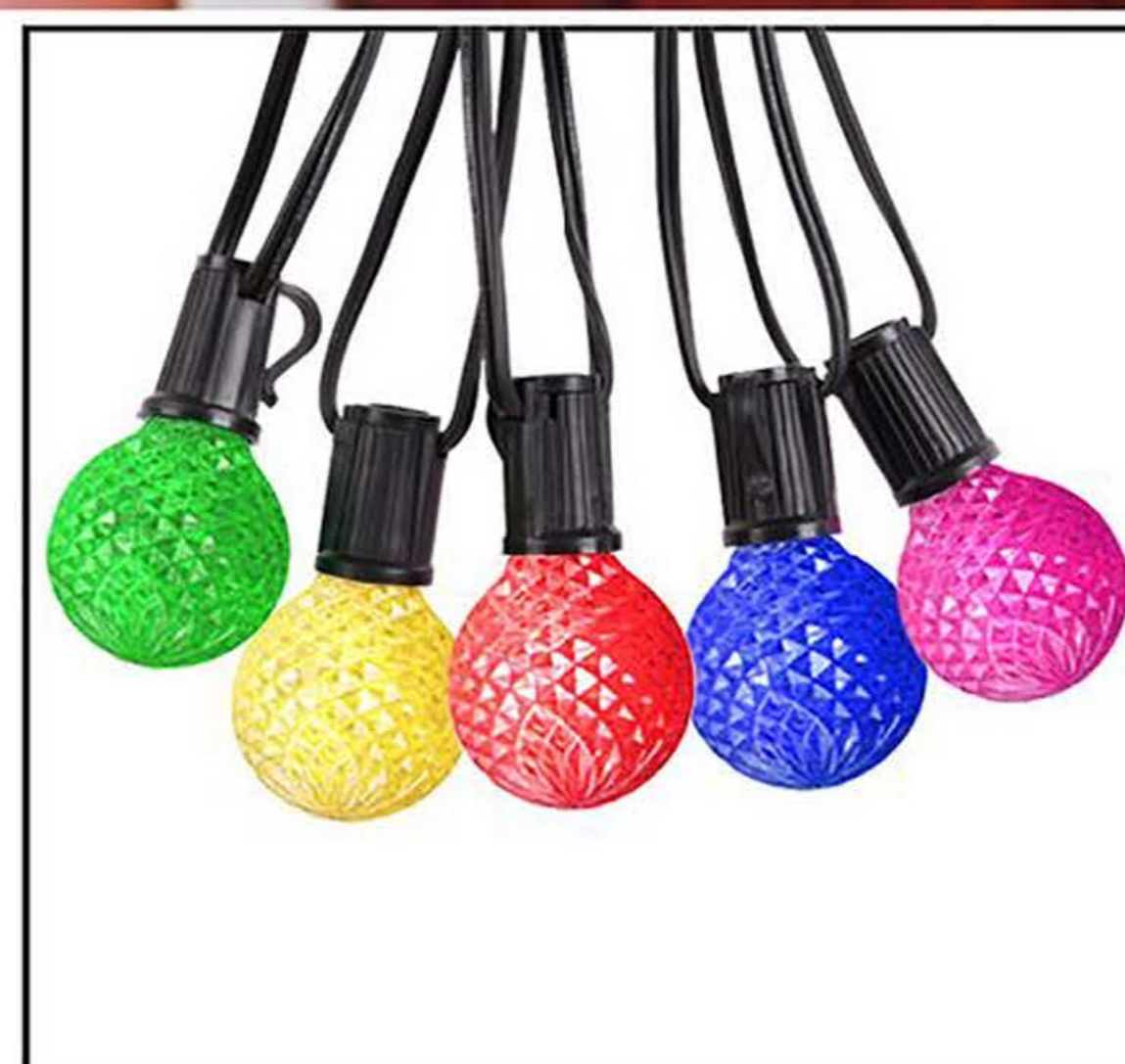
Product Model: LD-25-25FT-E12/G50/H-P/C/Mu-Multi color 25CT 25FT LED E12 G50 String Light- ( Plastic Multi color Blister starwberry/ Multi color Filament LED) Bulb Type Included: Filament LED Material: Plastic Base/Socket:E12 Power: 0.4W/Bulb Wire:SPT-1 20AWG/2C Black Wire Lamp distace:6"x12"x6" Voltage: 120V
