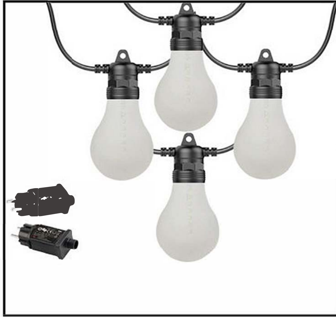
Product Model: LD-10-32.8FT-A60/F-P/C/C-Warm White-A 10CT 21.3FT LED A60 Low voltage decoration Flame Effect String Light(shape frosted Plastic Blister / Warm White SMD LED) Bulb Type Included: SMD LED Material: Plastic Power: A60 0.4W/Bulb(Warm White) Wire:VDE H05VV-F 0.5mm 2 /2C Black Wire Voltage: AC220-240V 5V 6W Function: 1.Flame effect;2.Always bright warm white
