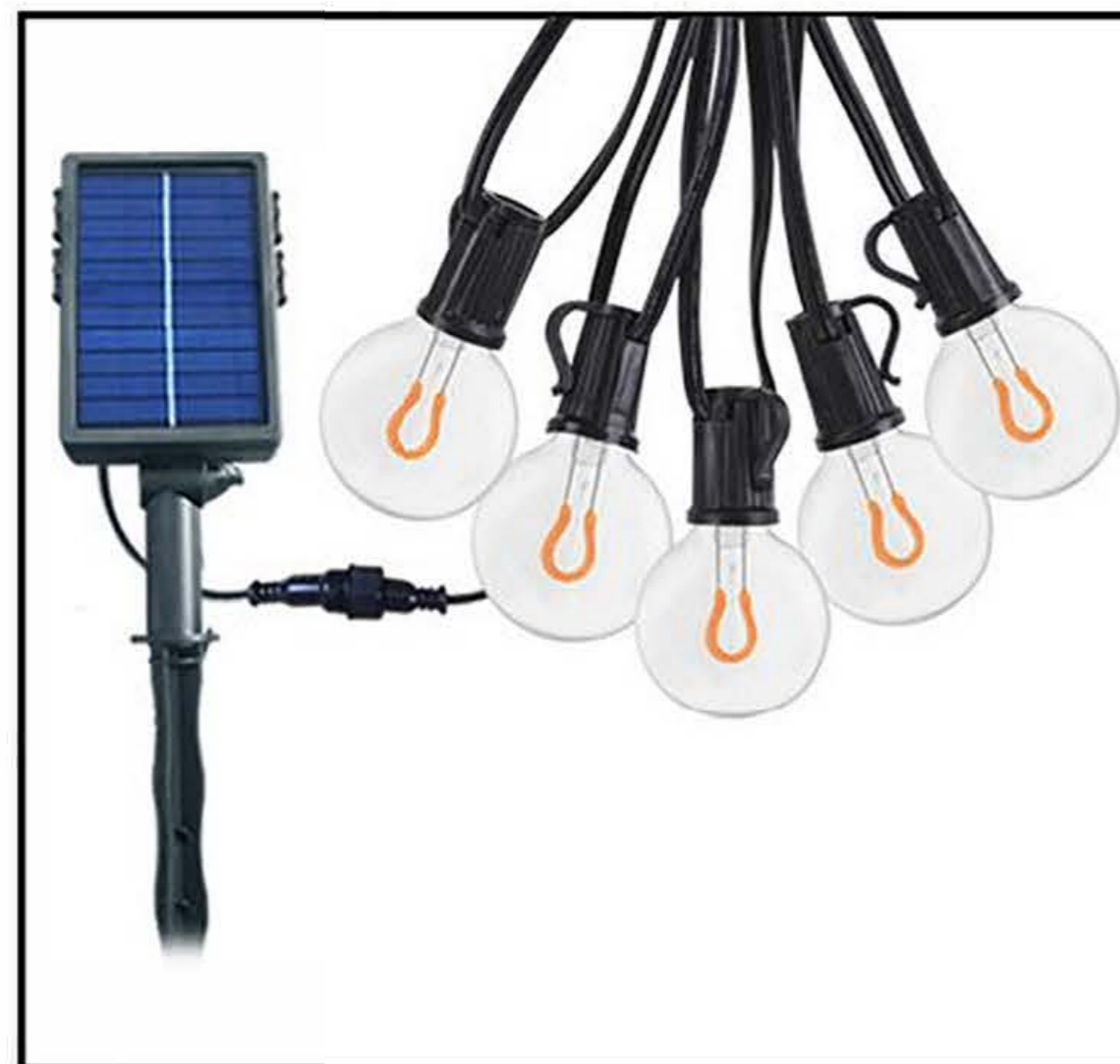
Product Model: LD-Solar-10-11FT-E12/G40/H-G/C/C-Warm White 10CT 11FT LED E12 G40 Solar/Battery Supply String Light- (Transparent Glass Blister/ Warm White Filament LED) Bulb Type Included: Filament LED Material: Glass Base/Socket:E12 Power: 0.4W/Bulb Wire:SPT-1 20AWG/2C Black Wire Voltage: 5.5V Dual power supply eight functions
