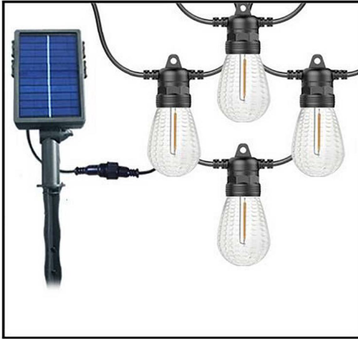
Product Model: LD-Solar-10-21.3FT-S14/L-P/C/C-Warm White-C 10CT 21.3FT LED S14 Solar/Battery Supply String Light- (Transparent Plastic Blister/ Warm White Filament LED) Bulb Type Included: Filament LED Material: Plastic Power: S14 0.4W/Bulb Wire:VDE H05VV-F 0.5mm 2 /2C Black Wire Voltage: 5.5V Dual power supply eight functions
