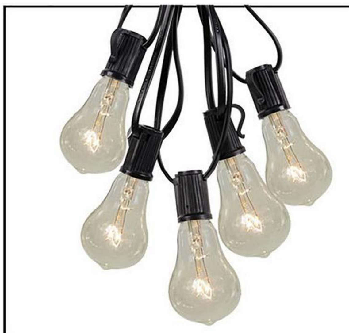
Product Model: LD-25-25FT-E17/PS50-G/C/C 25CT 25FT E17 PS40 Incandescent String Light- (Transparent Glass Blister/ Warm White Incandescent) Bulb Type Included: Incandescent Material: Glass Base/Socket:E17 Power: 7W/Bulb Wire:SPT-1 20AWG/2C Black Wire Lamp distace:6"x12"x6" Voltage: 120V
