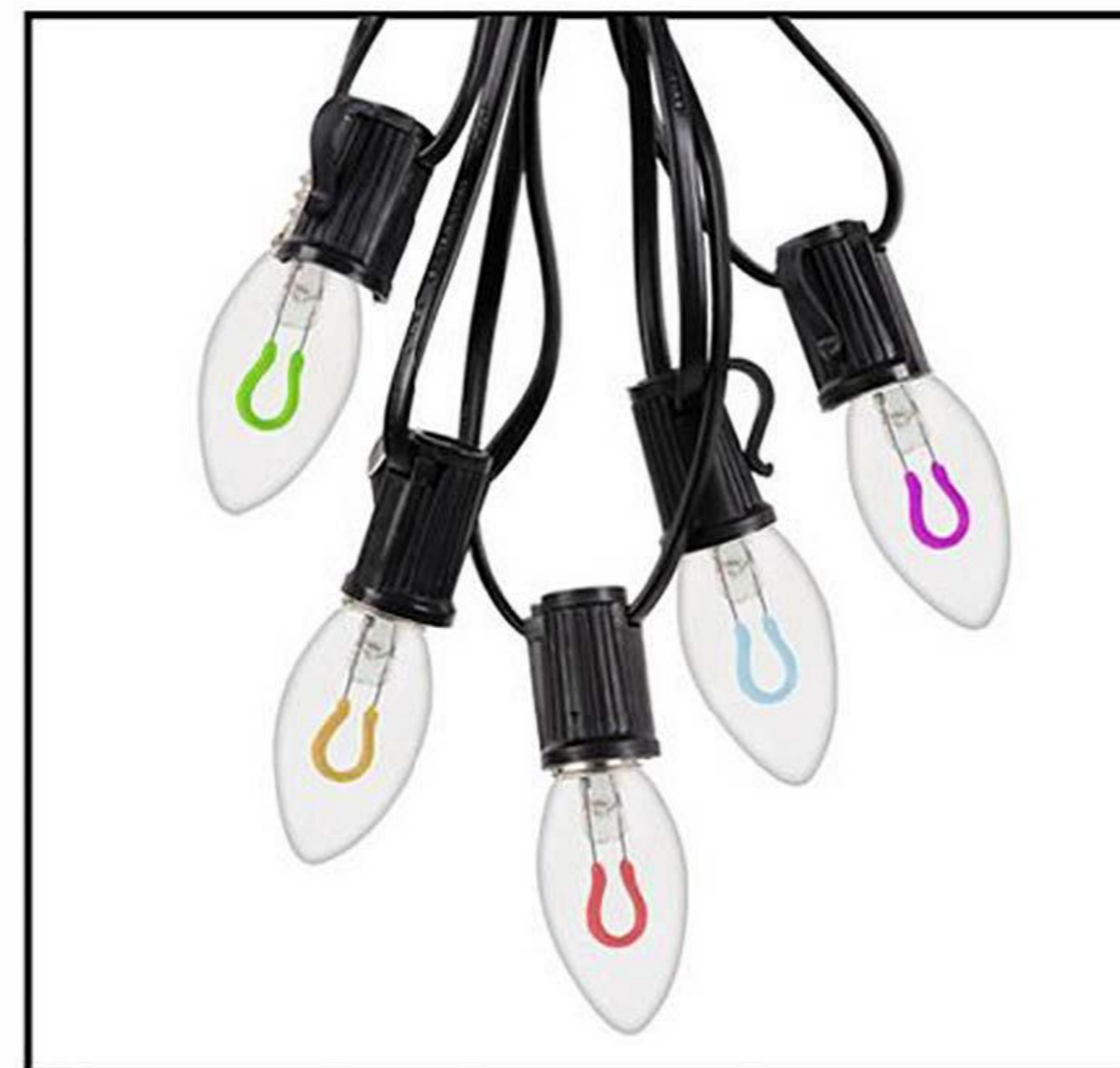
Product Model: LD-25-25FT-E12/C7/H-G/C/C-Multi color 25CT 25FT LED E12 C7 String Light- (Transparent Glass Blister/ Multi color Filament LED) Bulb Type Included: Filament LED Material: Glass Base/Socket:E12 Power: 0.4W/Bulb Wire:SPT-1 20AWG/2C Black Wire Lamp distance:6"x12"x6" Voltage: 120V
