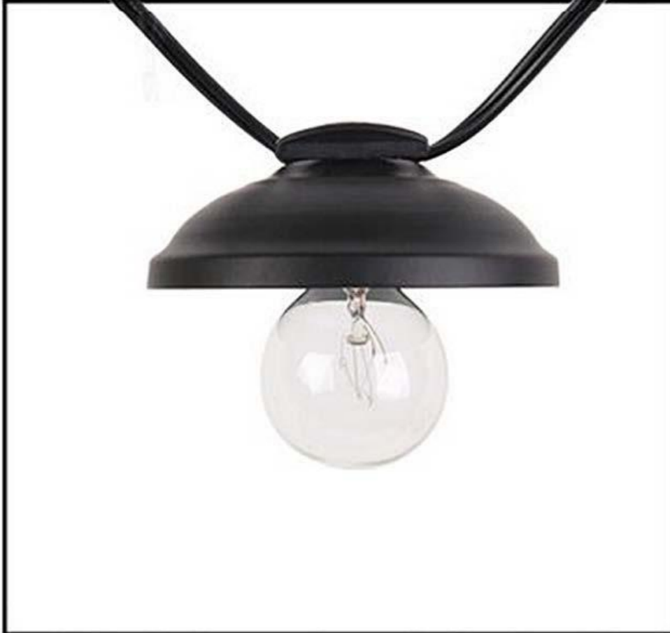
Product Model: LD-10CT-10FT-E12/G40-Modeling/13- Warm White 10CT 10FT E12 G40 Iron modeling garden String Light- (Transparent Glass Blister/ Warm White Incandescent) Modeling Size: \Phi 83mm*25mm Material: Glass/Metal Base/Socket:E12 Bulb: G40/10CT Bulb Type Included: Incandescent Wire:SPT-1 20AWG/2C Black Wire Lamp distace:6"x12"x6" Voltage: 120V
