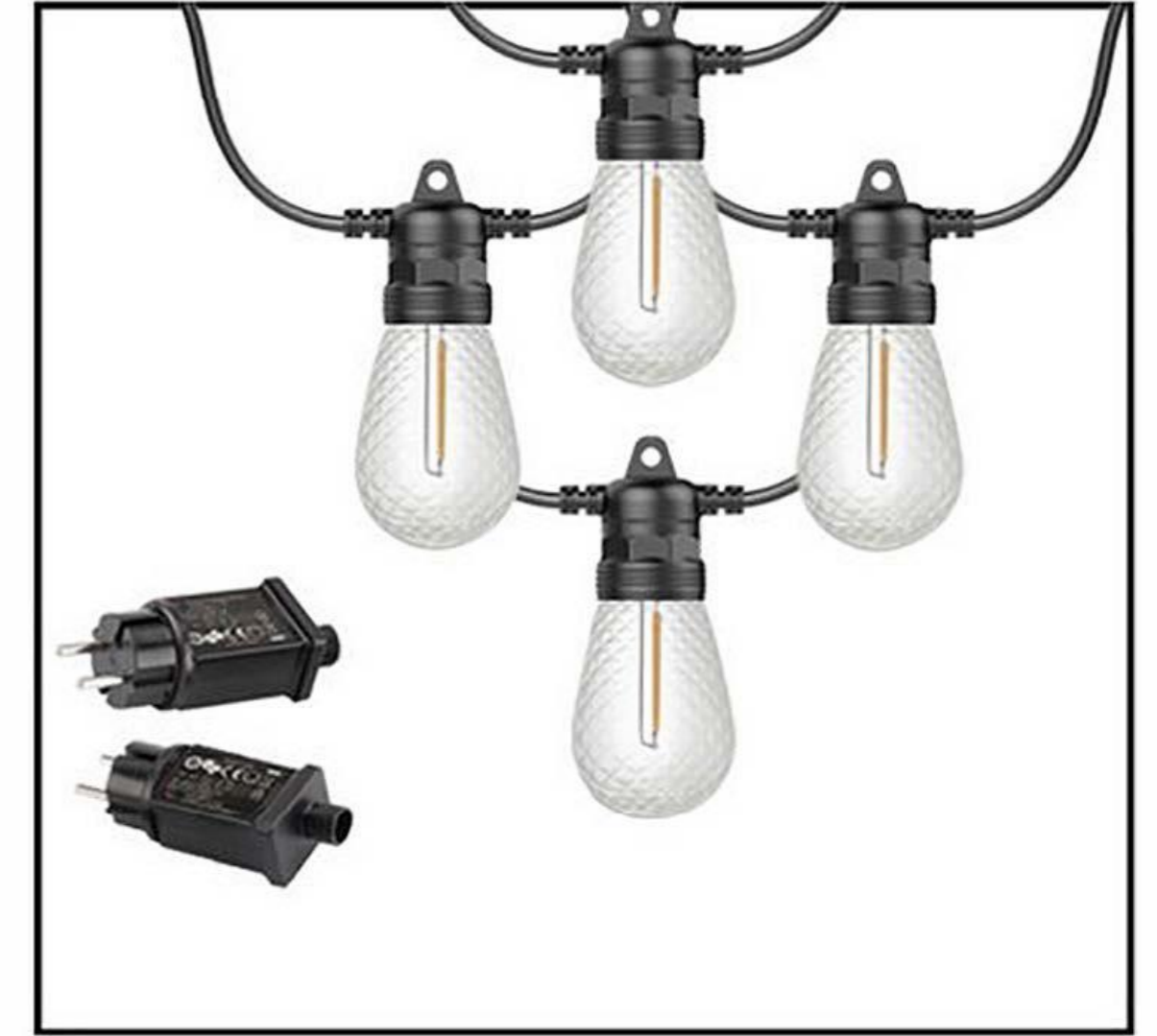
Product Model: LD-10-21.3FT-S14/L-P/C/C-Warm White-B 10CT 21.3FT LED S14 Low voltage decoration String Light- (Transparent Plastic Blister/ Warm White Filament LED) Bulb Type Included: Filament LED Material: Plastic Power: S14 0.4W/Bulb Wire:VDE H05VV-F 0.5mm 2 /2C Black Wire Voltage: AC220-240V 5V 6W Dual power supply eight functions
