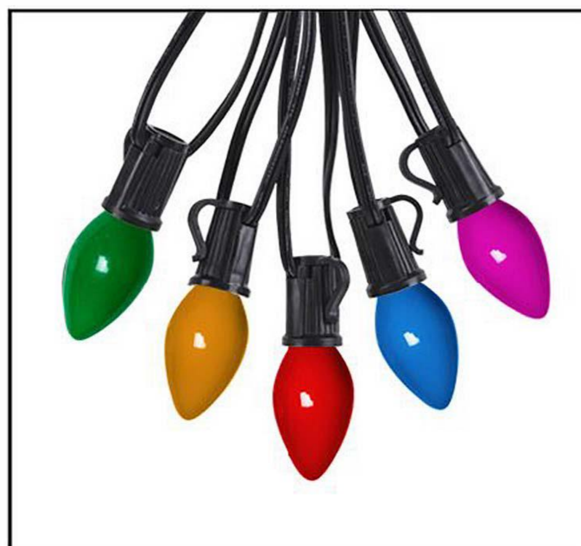
Product Model: LD-25-25FT-E12/C7/L-P/Mu-Warm White 25CT 25FT LED E12 C7 String Light (Transparent Plastic - Multi color Blister/ Warm White Filament LED) Bulb Type Included: Filament LED Material: Plastic Base/Socket:E12 Power: 0.4W/Bulb Wire:SPT-1 20AWG/2C Black Wire Lamp distace:6"x12"x6" Voltage: 120V
