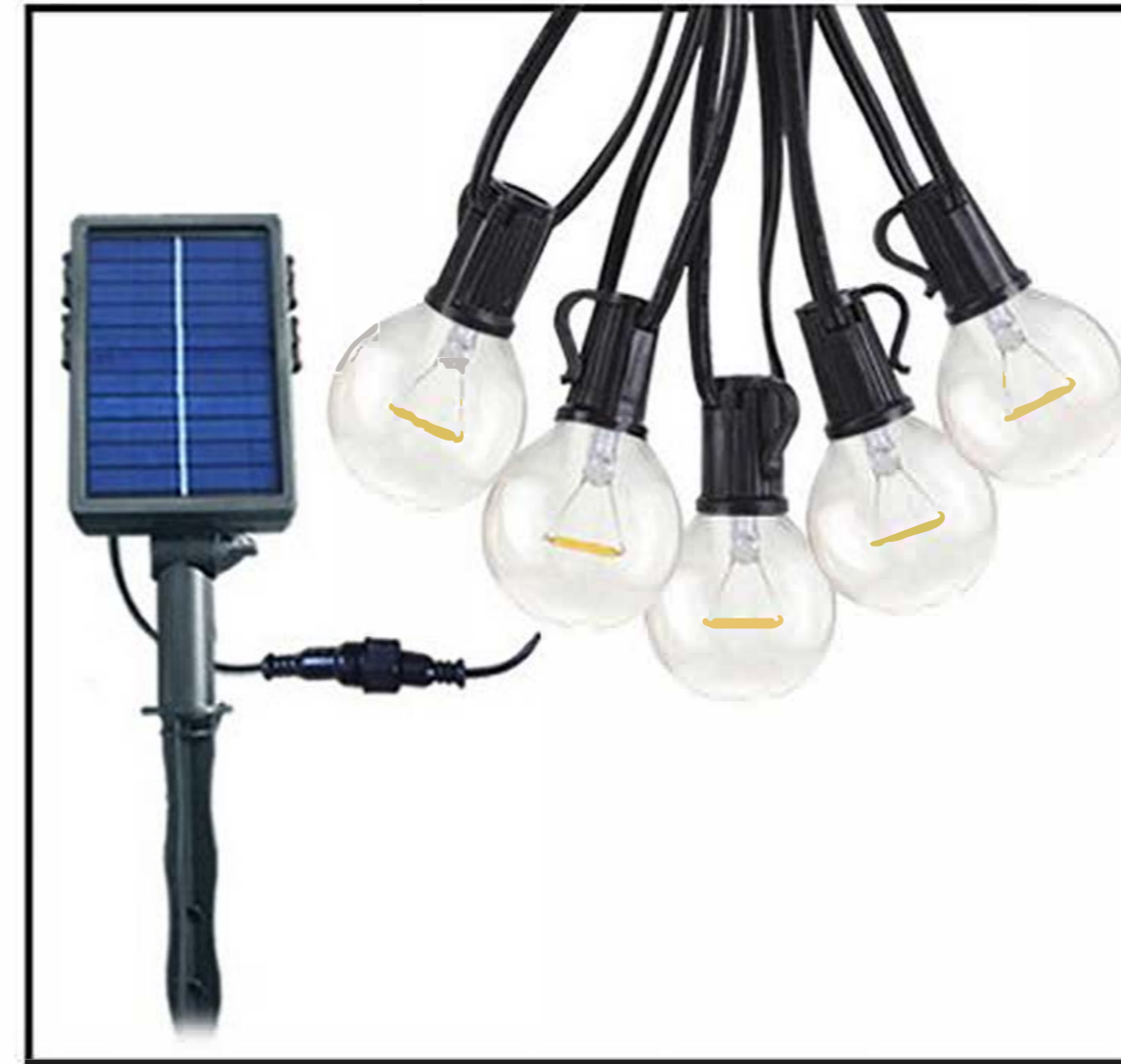
Product Model: LD-Solar-10-11FT-E12/G40/L1-G/C/C-Warm White 10CT 11FT LED E12 G40 Solar/Battery Supply String Light- (Transparent Glass Blister/ Warm White Filament LED) Bulb Type Included: Filament LED Material: Glass Base/Socket:E12 Power: 0.4W/Bulb Wire:SPT-1 20AWG/2C Black Wire Voltage: 5.5V Dual power supply eight functions
